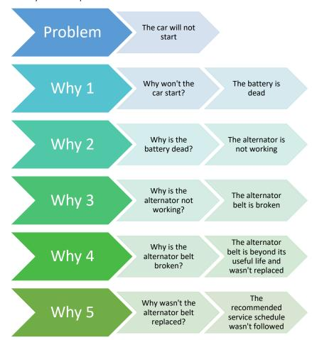
Therefore the root cause for the vehicle not starting was not as appeared on first sight, that the battery was dead, but because the vehicle was not serviced according to the schedule.
